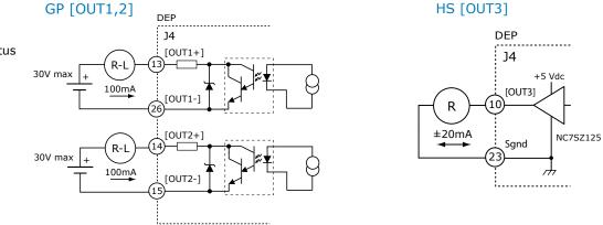
When configured as a Custom function, the output will go active when any of the events becomes true. When active, the output can be configured as on or off. The output can also be set to latching, or non-latching.
